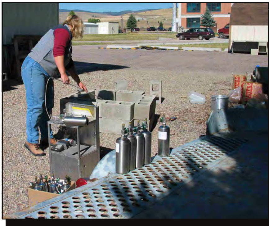
Figure 2—Using canisters to collect gas samples from a simulated campfire for analysis with a gas chromatograph-mass spectrometer.
